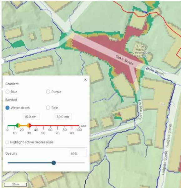
Figure 6 – Duke St: Depression Storage. Max Depth: 65cm, Volume: 250m 3
