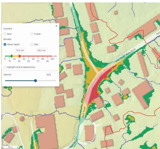
Figure 13 - Depression Storage. Max Depth: 65cm, Volume: 680m 3
